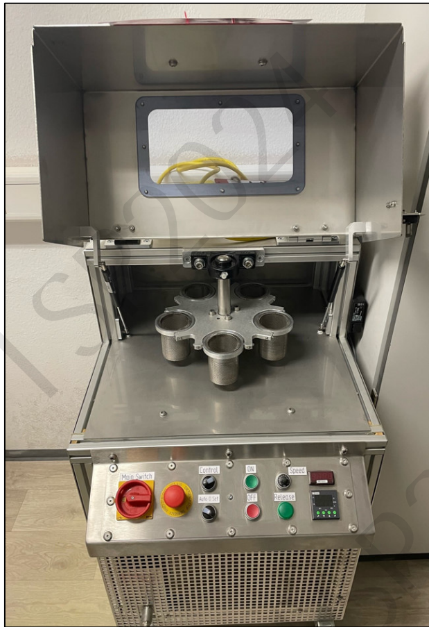
Fig. 2: Centrifuge (spin dryer) built at the RHI Magnesita Technology Center Leoben, Austria.
